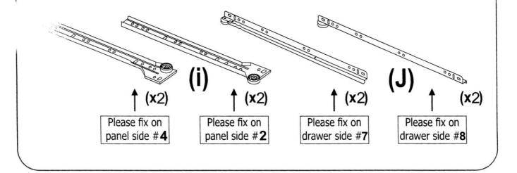
02 The wheel to the front! The wheel to the H front! H PRE-DRILLED HOLES H H H H Right side (+) SPACE (+) BACK SPACE (-) BOTTOM Division / left side Qty **Drawer Runner 350mm**
